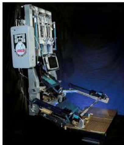
advanced Resistive Exercise Device (aRED)
